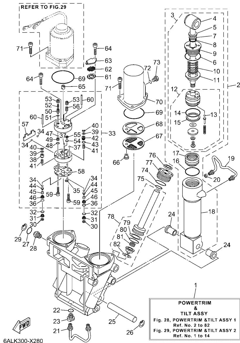
**FIG. 28 POWER TRIM & TILT ASSY 1** **COMPOSER Y PODER VARILLA 1**
